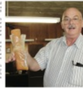
Russell Pate holds a rusty filter he said had been in the system for only nine days.
